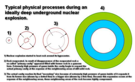
4) Final picture. White: the underground cavity (its secondary size); blue: a so-called "crashed zone"- totally pulverized rock (crashed into complete microscopic dust ~ 100 micron particle size); green: a so-called "damaged zone"- partly crashed rock.
